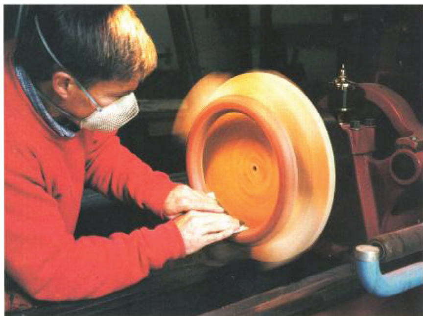
■ Metal lathe fitted with a fixture using reversible wooden jaws to hold the work.
