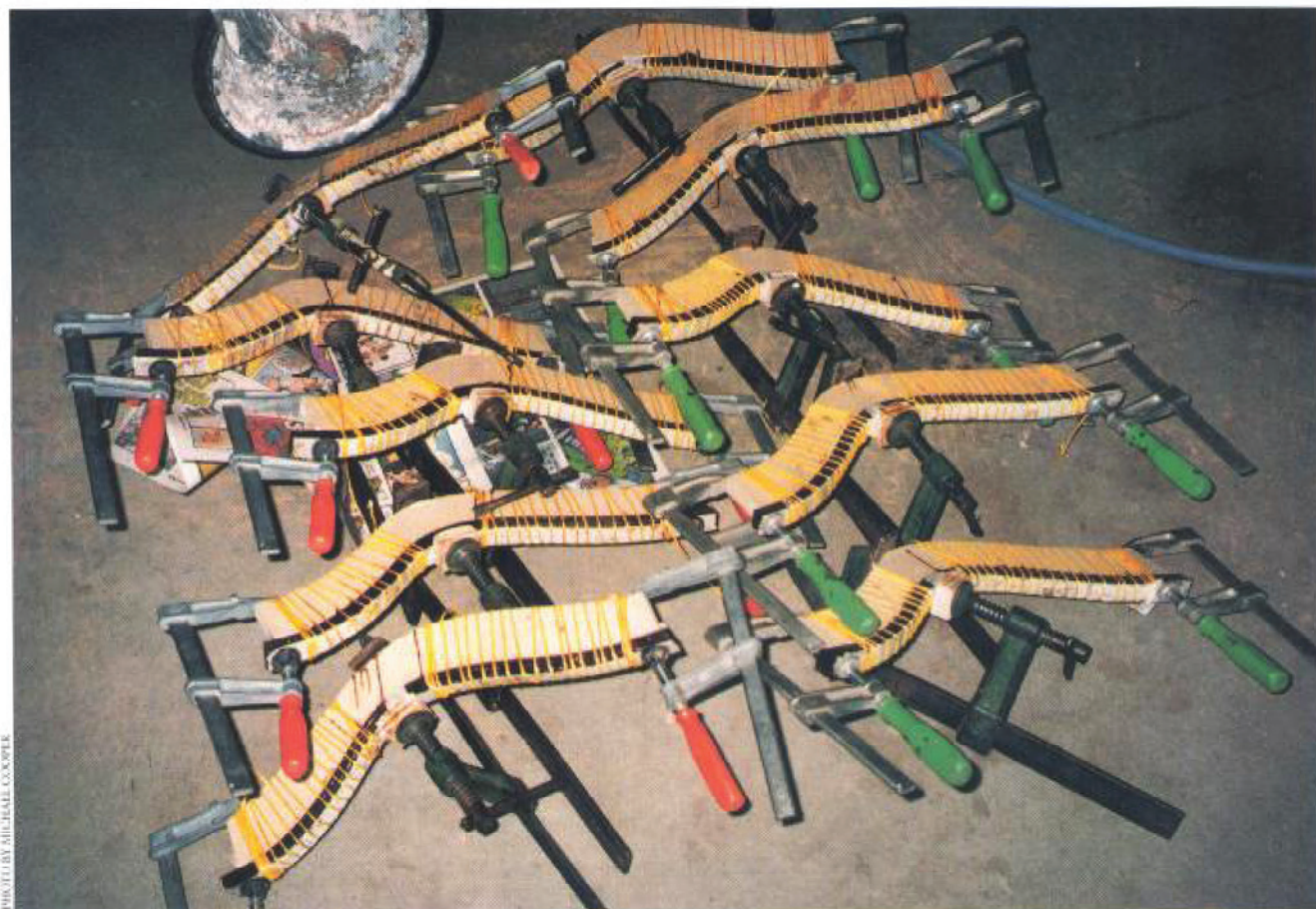
■ A multitude of clamps and forms are used to create some of the many components used in just one piece.
